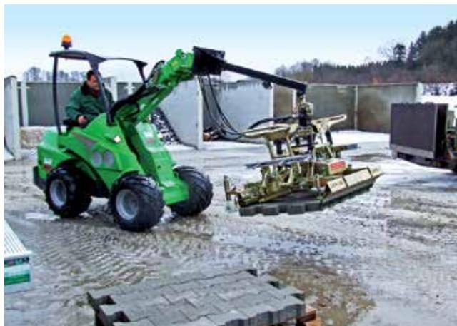
Installation clamp in combination with Mini-excavator
