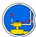
In order to connect the forklift truck and the fork sleeve (3), the forklift truck forks (1) are inserted into the fork sleeve (3).
