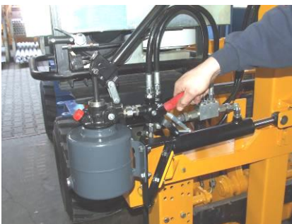
Move the red lever in Position B
