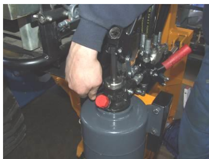
Move lever (at the hand pump) in Position II .
