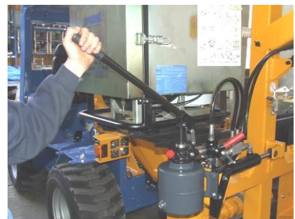
Operate the lever at hand pump to move the mast to the right.
