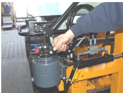
Move the red lever in Position A
