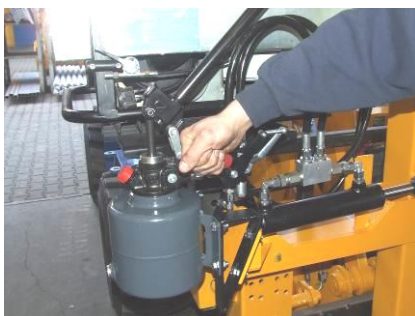
Move the red lever in Position A
