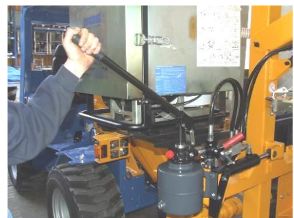
Operate the lever at hand pump to move the mast to the left.
