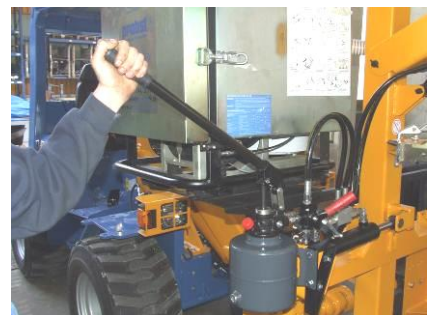
Operate the lever at hand pump to move the mast upwards.
