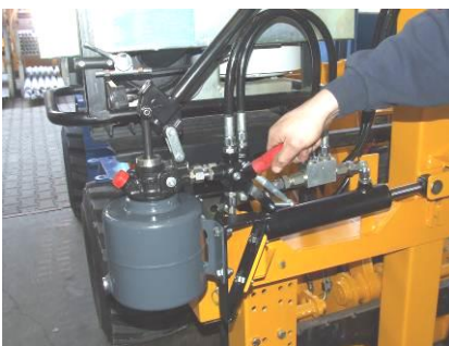
Move the red lever in Position B
