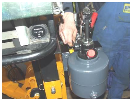
Move lever (at the hand pump) in Position I
