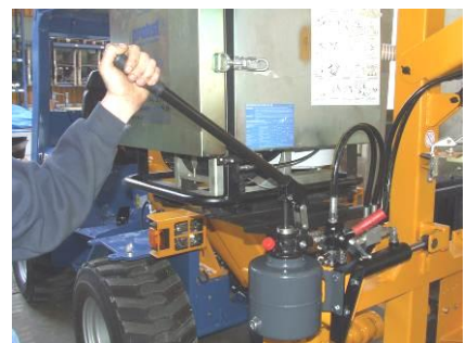
Operate the lever at hand pump to move the mast downwards.
