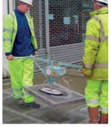
Flexible and powerful – for nonporous materials such as granite or concrete parts up to 150 kg. With battery drive. Order-No. 52710008
