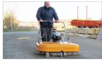
With the EF-H-GREENLINE electric paver jointing device, the application of jointing material (dry or with water addition) is fast, quiet and emission-free.
