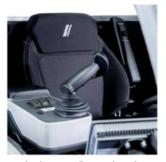
Joystick with ergonomically arranged controls
