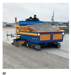
Sideways foldable chutes to avoid that material is spilling over the side of the hopper. Two independently hydraulically operated lids at the bottom of the hopper to perfectly control the material flow.
