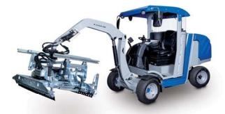
Equipped with partially enclosed operator's cabin, adjustable standard seat with mechanical suspension, 2.4" screen and standard boom.
