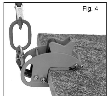
Plate in horizontal position: position clamp in the centre of the plate above the centre of gravity and the narrow jaw must show downwards. Open clamp against the spring tension and push in to the limit stop (Fig. 4). Now lift plate for approx. 10 cm.
