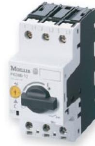
A motor protection switch is used when a vacuum blower or a vacuum pump is used. The motor protection switch serves to switch off the vacuum generator and simultaneously protects it. The motor protection switch is designed for the connected vacuum generator. No further consuming devices may be connected to the outlet of the motor protection switch.
