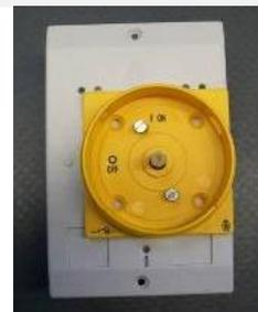
2. Screw the mounting frame cover onto the switch. Screw through the yellow mounting plate of the main switch. Use the marked holes (2) in the cover for this. The Glöckner Möller logo (1) can be used as an orientation aid.
