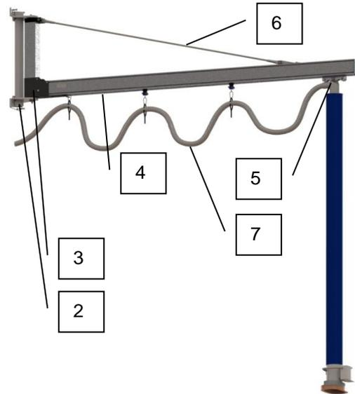
2.1.3 Column-mounted jib crane with flat jib
