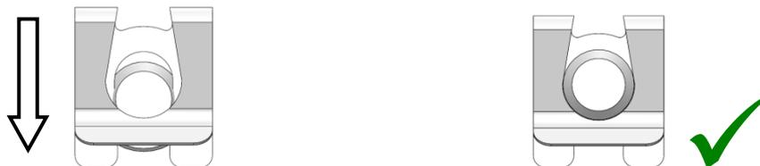
For a bolt diameter of 12 => use size 12mbo08 (No. 20.06.04.00036)
