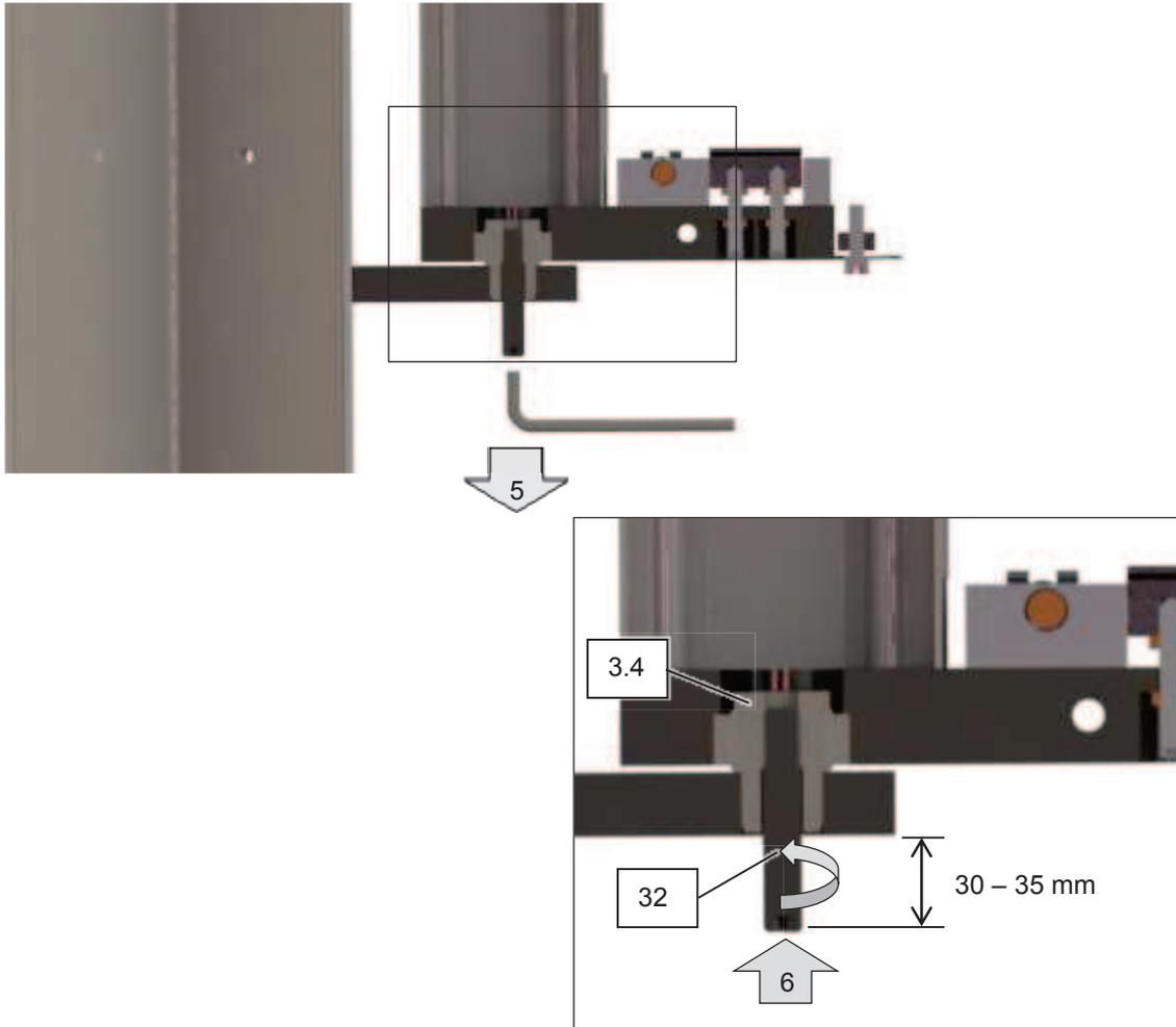
5. Pull the bolt (3.4) down through the hole of the lower bearing plate (1.2) using the set screw (32).
