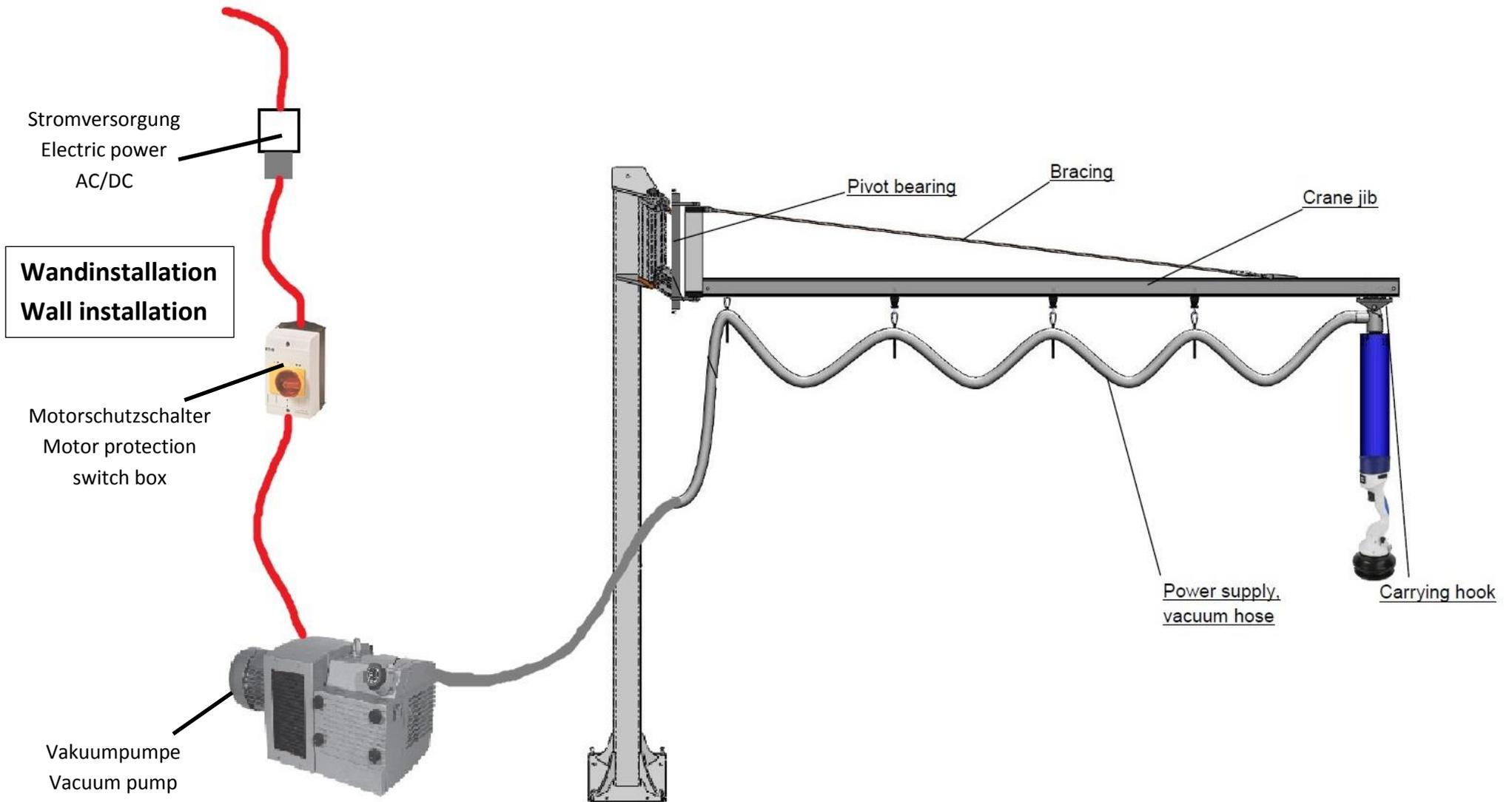
Installation Motorschutzschalter (Kransäule) / Installation of motor protection switch box at the swing crane by drilling of mounting holes in the column.
