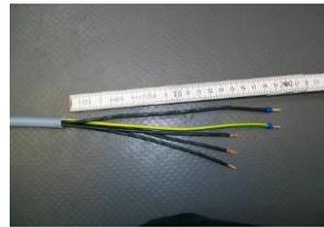
2. Pull the cables through the opening and prepare them for connection. Stripping around 25 cm of the cables is recommended.
