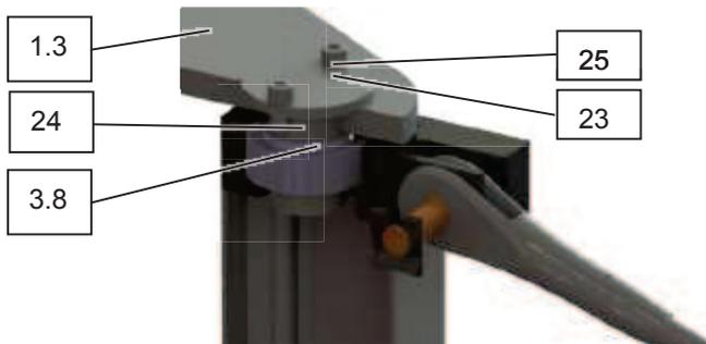
1. Insert the upper bolt (24) through the hole in the upper bearing plate of the wall bracket / crane column (1.3) and in the upper bearing (3.8) of the pivot bearing.
