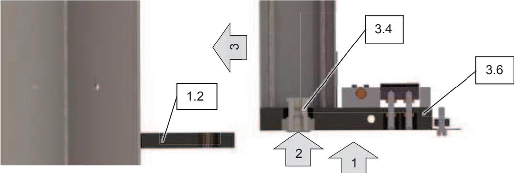
1. Lift the crane jib with appropriate hoist to the height of the lower bearing plate of the wall bracket / crane column (1.2).
