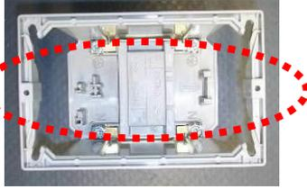
6. Install additional neutral terminal on the mounting frame. As with the grounding terminal, this terminal is only pressed in from the side.
