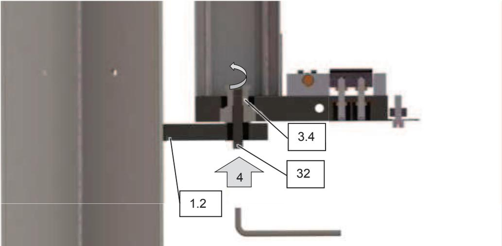
4. Screw the set screw (32) 10 mm into the bolt (3.4) from below through the lower bearing place of the wall bracket / crane column (1.2).
