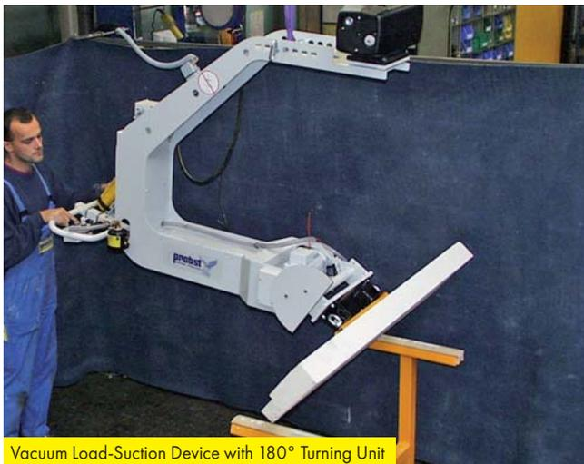
Vacuum Load-Suction Device with 180° Turning Unit
