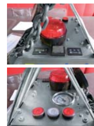
Panel de mando SM-600-GREENLINE-POWER
